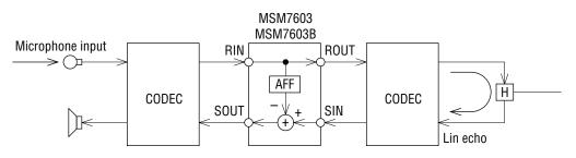
Example 3: Canceling of both acoustic and line echo (to handle both acoustic echo from line input and line echo from microphone input)
