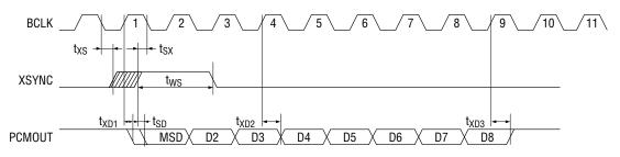
When  $t_{XS} \leq 1/2$  • Fc, the Delay of the MSD bit is defined as  $t_{XD1}.$  When  $t_{SX} \leq 1/2$  • Fc, the Delay of the MSD bit is defined as  $t_{SD}.$
