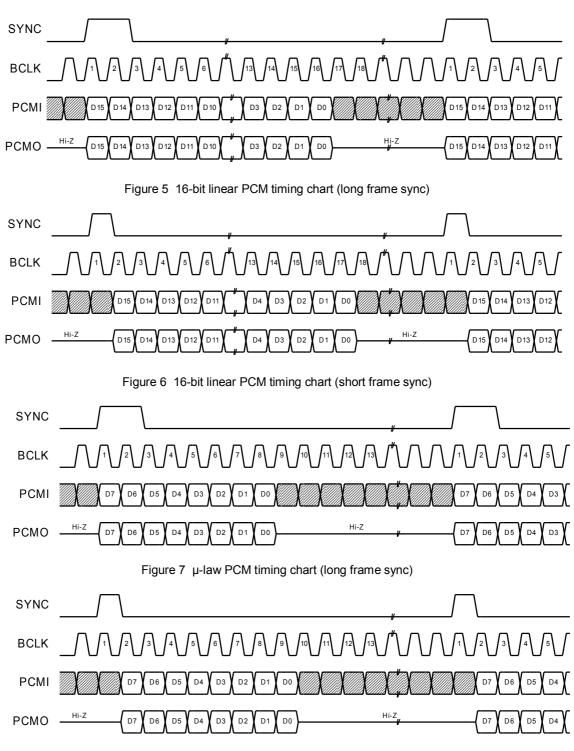
Figure 8 µ-law PCM timing chart (short frame sync)
