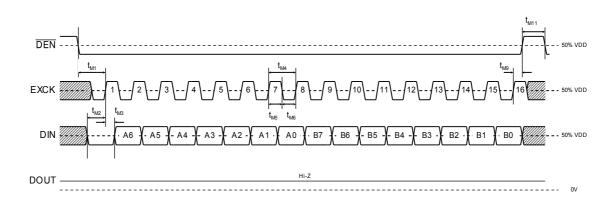
Figure 19 Write Timing
