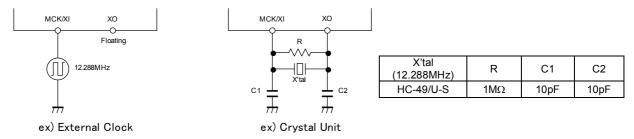
Figure 4 Examples of external clock and crystal unit as a master clock
