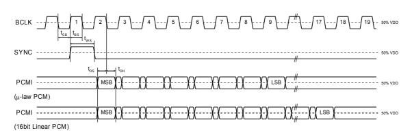
Figure 16 PCM Input Timing (Short Frame Sync)
