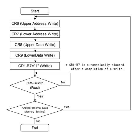
Figure 26 Internal Data Memory Access Flow Chart
