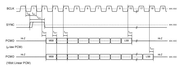
Figure 18 PCM Output Timing (Short Frame Sync)
