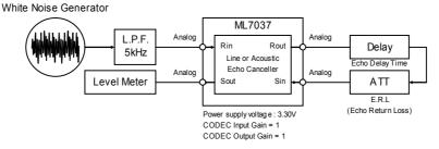
Figure 22 Measurements (Echo Attenuation)
