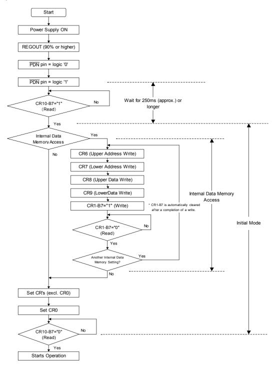
Figure 25 Micro Controller Interface Flow Chart
