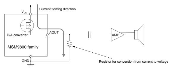
Circuit connection between the MSM9800 family product and amplifier IC
