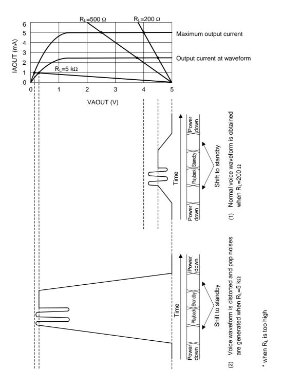
Relationship between AOUT pin voltage and AOUT output current at  $V_{DD} = 5 \text{ V}$
