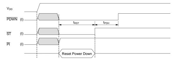
Note: A level input in combination of  $\overline{PDWN}="L"$ ,  $\overline{ST}="L"$  and  $\overline{Pl}="H"$  resets the LSI. After Power-On, you need to do an initial reset as shown in the above chart.
