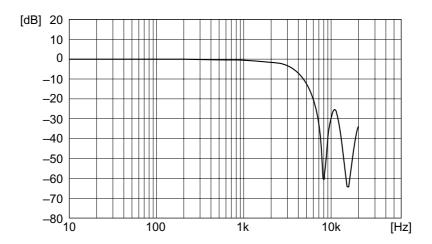
Figure 6 LPF Frequency Characteristics (f<sub>SAM</sub>=8 kHz)
