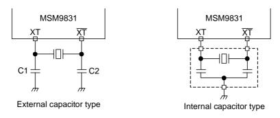
Figure 4 Oscillation Circuit with an external ceramic oscillator
