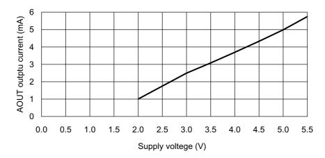
Relationship between supply voltage and AOUT output current (Ta =  $20^{\circ}$ C, VAOUT =  $V_{DD}$ , PCM at maximum)
