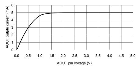
Relationship between AOUT pin voltage and AOUT output current (Ta = 25°C,  $V_{\rm DD}$  = 5.0 V, PCM at maximum)
