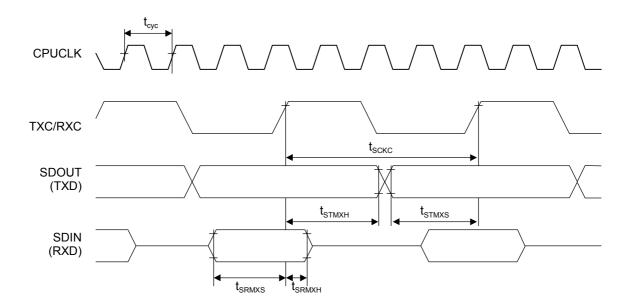
Slave mode (Clock synchronous serial port)
