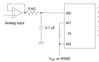
Cross talk is the difference between the A/D conversion results when the same analog input is applied to Al0 through Al3 and the A/D conversion results of the circuit to the left.
