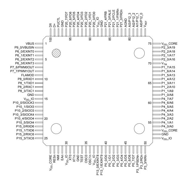
100-pin Plastic TQFP
