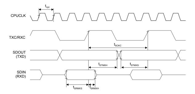
Slave mode (Clock synchronous serial port)
