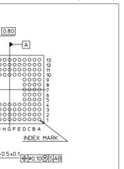
Ф0.20SB 11.0 ⊕0.20SA 0.7 В 11.0 ×4 0.15 0.7 INDEX MARK \$\phi 0.5 \pm 0.10 \mathred{\text{M}} \square \phi 0.10 \mathred{\text{M}} \square \text{AB} // 0.20 S 0.10 S Package material Epoxy resin Sn/Pb Ball material Package weight (g)
